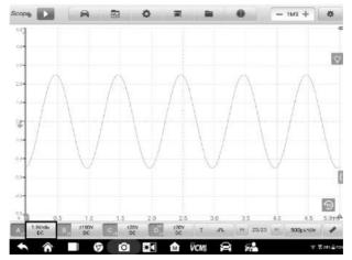
Figure 7-52 Sample Amplitude Setting Screen (DC 1.0V/div)
