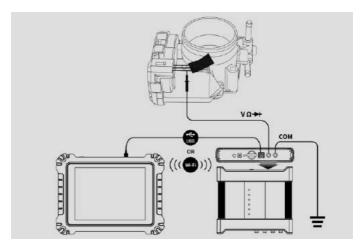
Figure 7-1 Sample Connection Diagram
