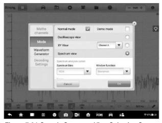
Figure 7-84 Sample Spectrum View Selection Screen
