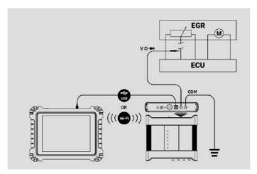
Figure 7-1 Sample Connection Diagram
