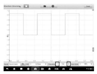
Figure 7-20 Sample Frequency Setting Screen 1
