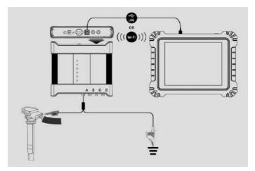
Figure 7-1 Sample Connection Diagram
