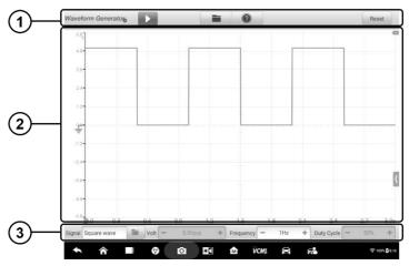
Figure 7-4 Sample Waveform Generator Menu Screen
