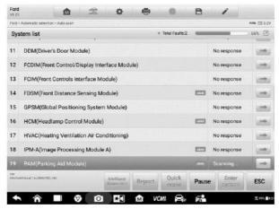
Figure 5-5 Sample Fault Scan on System List Screen 2
