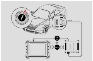
Figure 7-60 Sample DLC Connection Diagram
