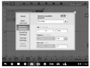
Figure 7-21 Sample Waveform Generator Setting Screen
