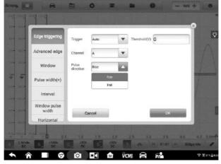
Figure 7-68 Sample Pulse Direction Screen
