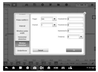
Figure 7-75 Sample Window Distortion Settings Screen
