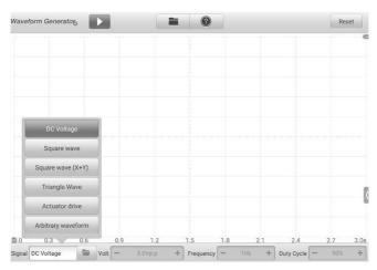
Figure 7-10 Signal Mode Setting Screen
