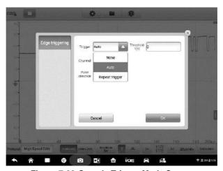
Figure 7-23 Sample Trigger Mode Screen
