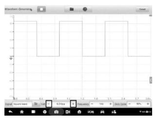
Figure 7-17 Sample Voltage Setting Screen 1
