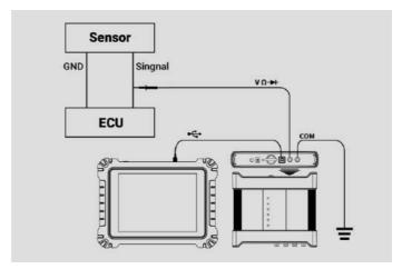
Figure 7-16 Sample Arbitrary Waveform Connection Diagram
