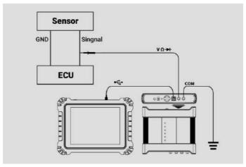
Figure 7-15 Sample Triangle Waveform Connection Diagram
