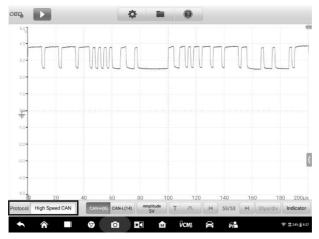
Figure 7-16 Sample Protocol Type Button Screen
