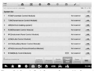
Figure 5-4 Sample Fault Scan on System List Screen1
