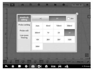
Figure 7-49 Sample Amplitude Setting Screen (DC 5V)
