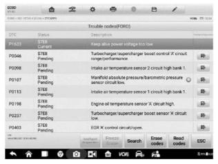
Figure 4-29 Sample DTC & FFD Screen
