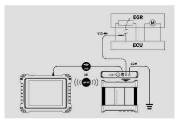
Figure 7-11 Sample DC Voltage Connection Diagram
