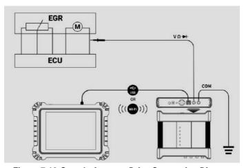
Figure 7-12 Sample Actuator Drive Connection Diagram
