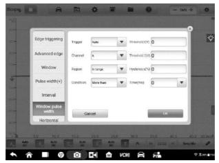
Figure 7-73 Sample Window Pulse Width Settings Screen
