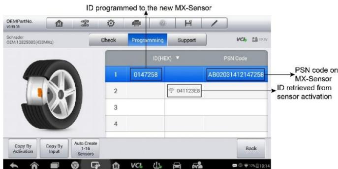
**Figure 4-34 Sample Programming Screen via OEM Part No.**
