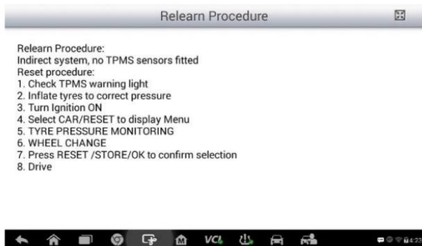
**Figure 4-6 Sample Relearn Procedure for Indirect TPMS**
