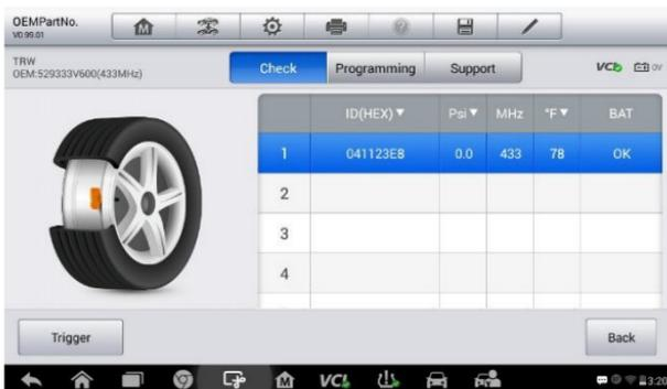
**Figure 4-33 Sample Check Screen via OEM Part No.**
